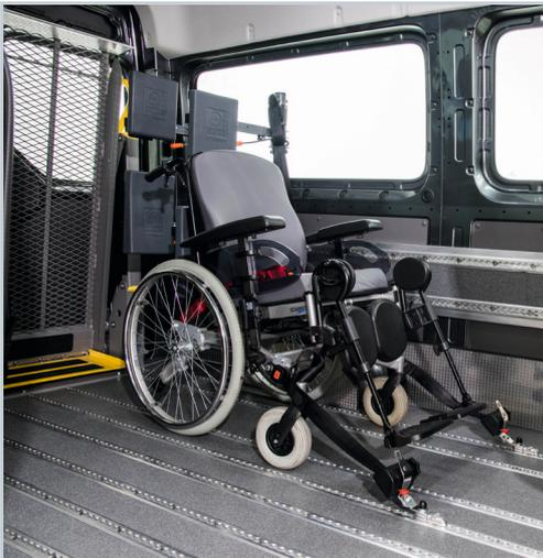
The wheelchair enters the vehicle via lift. AMF-Bruns PROTEKTOR system for wheelchair and occupant restraint.
