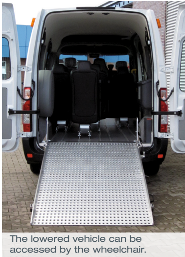
Vehicle with folded ramp. Rear view is maintained.
