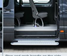
Step and grab handle on the side entry allow comfortable access to the passenger cabin.
