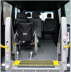
With a lift, the wheelchair gets access to the vehicle. The AMF-Bruns restraint system secures wheelchair and occuppant.
