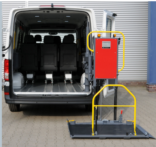
Lowered lift, ready for wheelchair access.
