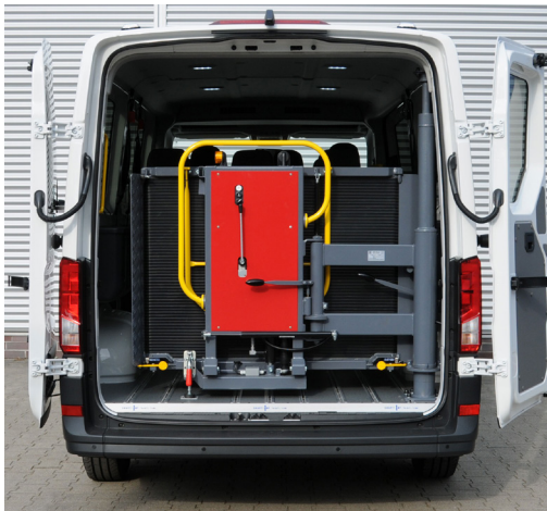
Swivel lift folded back in a space-saving way.
