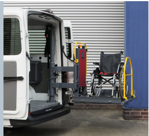
The AMF-Bruns swivel lift BSL 350 in lifting operation.
