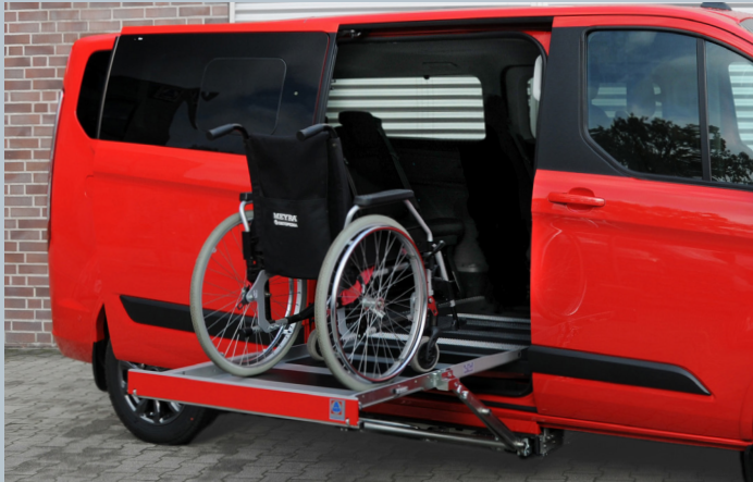
The automatic roll-off safety barrier and the generous platform provide additional security.
