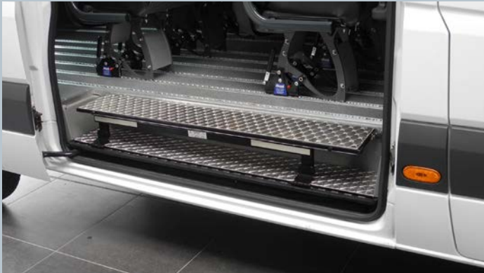
Fold-out step on same level as vehicle floor
