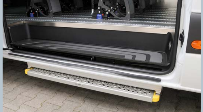
Step in stowed position fitted under the vehicle
