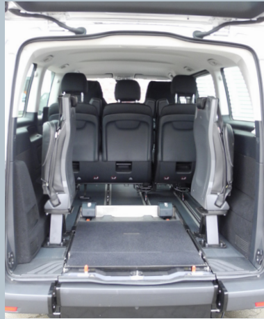
With the optional EASYFLEX ramp folded down the luggage compartment is fully usable.
