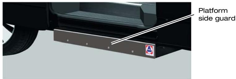
Figure 9: Cassette Lift K90 ACTIVE, Retracted
