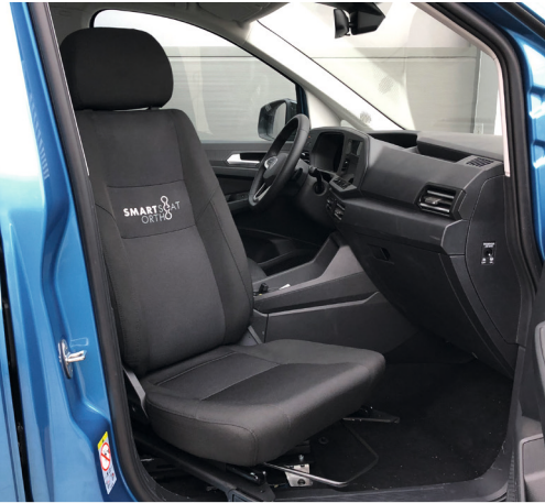
With its flat seat cushion, the Smartseat Ortho enables easy moving from the wheelchair into the vehicle.
