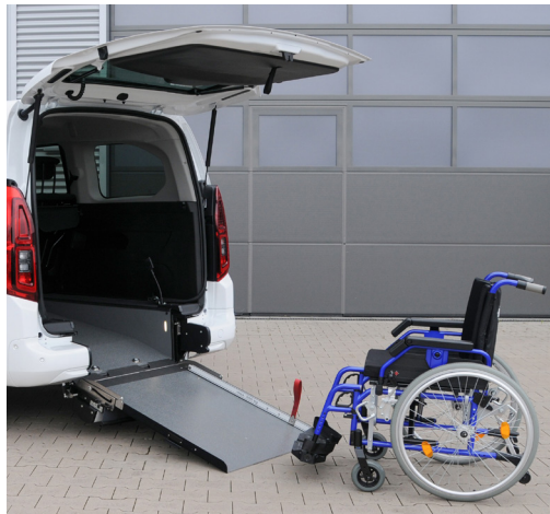
With the unfolded ramp the vehicle can be accessed comfortably with a wheelchair.
