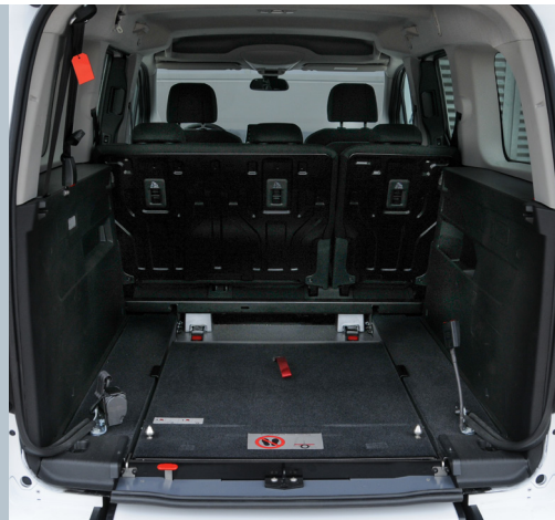
Optional EASYFLEX ramp folded flat allows full use of the luggage area.
