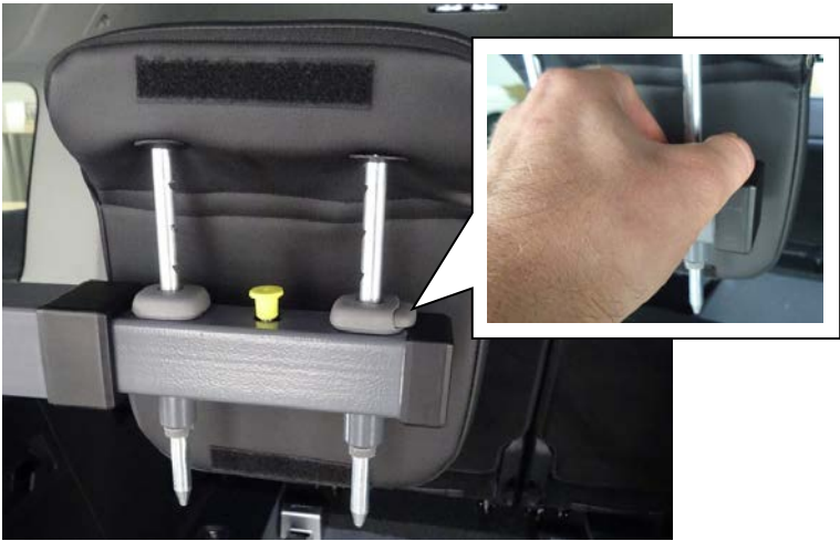
Figure 11: Press Height Unlatching Button
