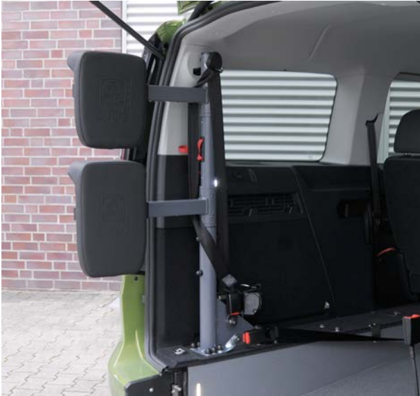
Figure 5: Swivel Arms Pivoted Towards the Rear
