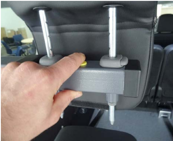
Figure 8: Press Lateral Unlatching Button
