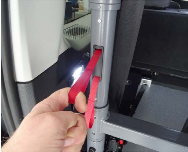
Figure 7: Pull Operating Strap (Here: Head Support Swivel Arm)
