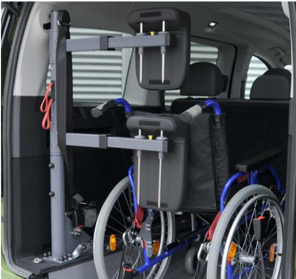
Figure 6: Swivel Arms in Position Behind the Wheelchair
