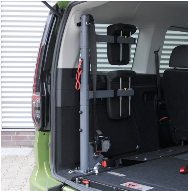
Figure 4: Swivel Arms Pivoted Towards the Front
