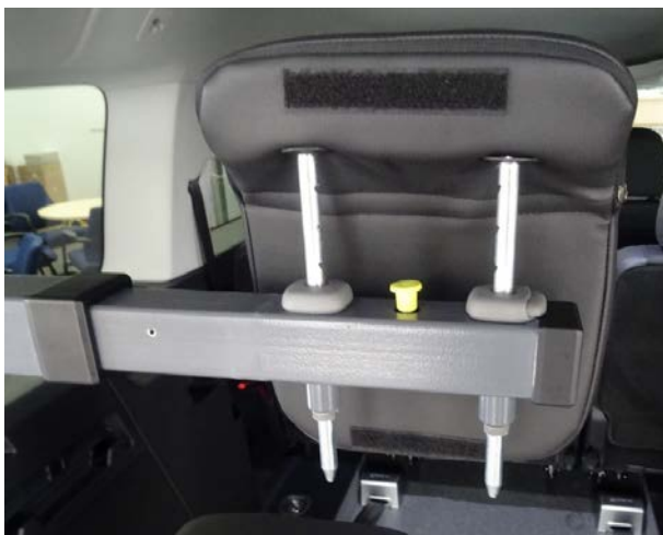
Figure 9: Swivel Arm, Extended
