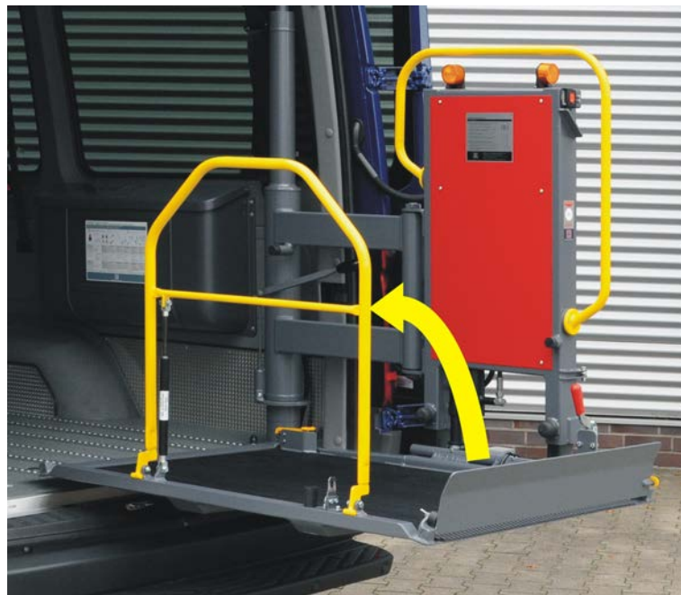
Figure 13: Raising the Side Guard Rail
