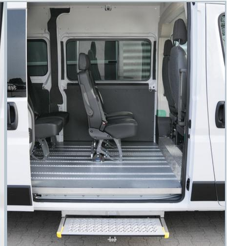
Electric step and handle on the side entry provide easy access to the passenger compartment.
