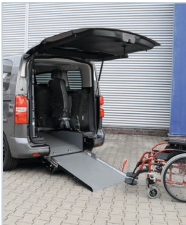
With the unfolded ramp the vehicle can be accessed comfortably with a wheelchair.
