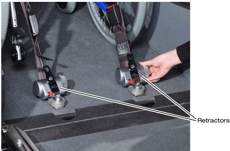
Figure 17: Tensioning the Retractors
