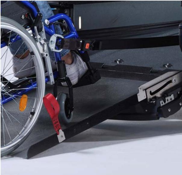
Figure 16: Electrically-Operated Belts Attached to the Wheelchair
