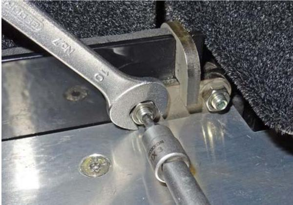
Figure 26: Adjusting the Play by Means of the Adjuster Screws
