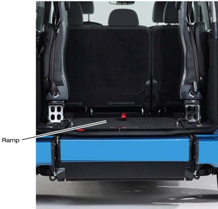
Figure 3: Fully Stowed EasyFlex Ramp
