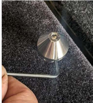
Loosening the clamping screw
