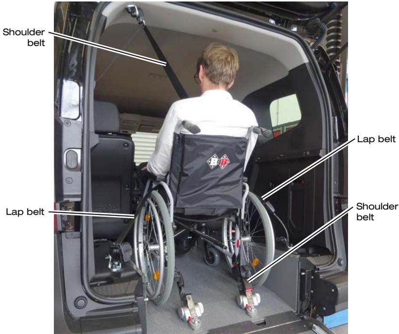
Figure 19: Fastening the Vehicle's Own Black Lap Belt and Shoulder Belt
