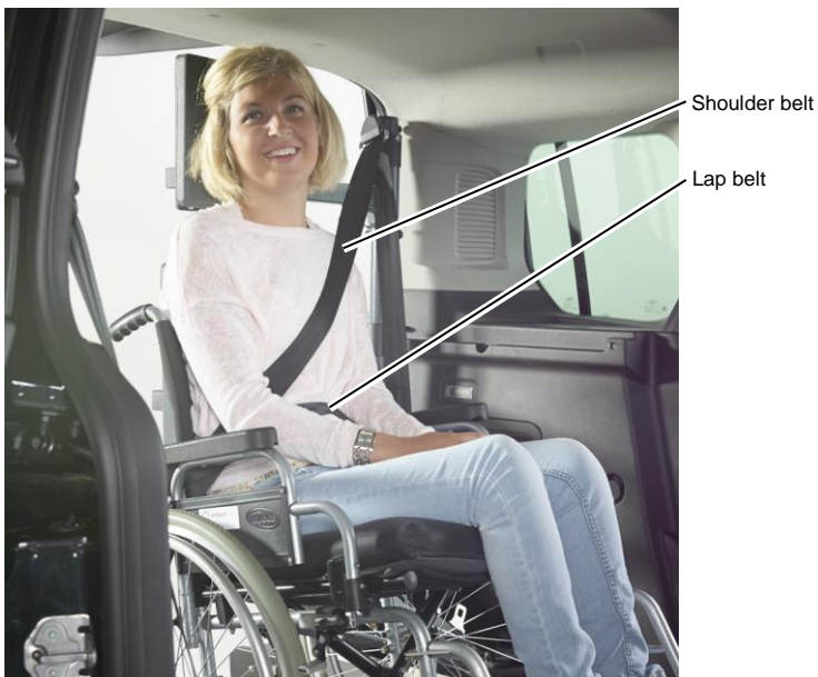
Figure 15: Safety Belts on the Passenger (1)
