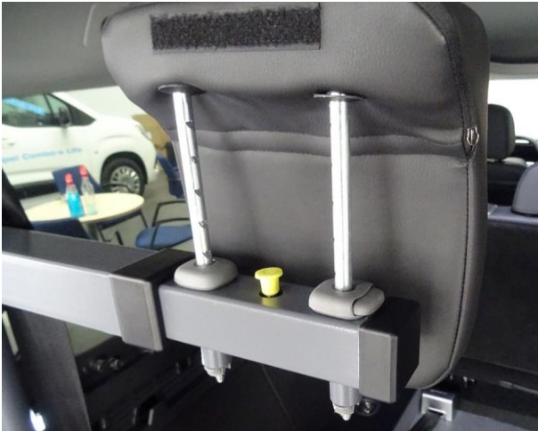
Figure 10: Head Support at the Maximum Height
