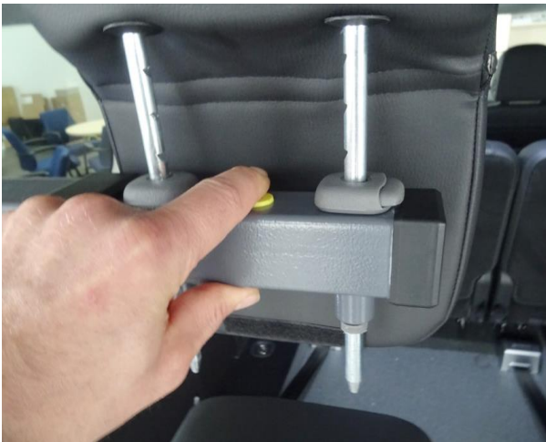
Figure 8: Press Lateral Unlatching Button
