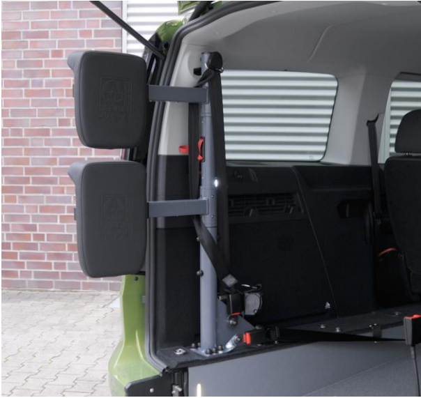
Figure 5: Swivel Arms Pivoted Towards the Rear
