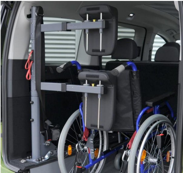
Figure 6: Swivel Arms in Position Behind the Wheelchair
