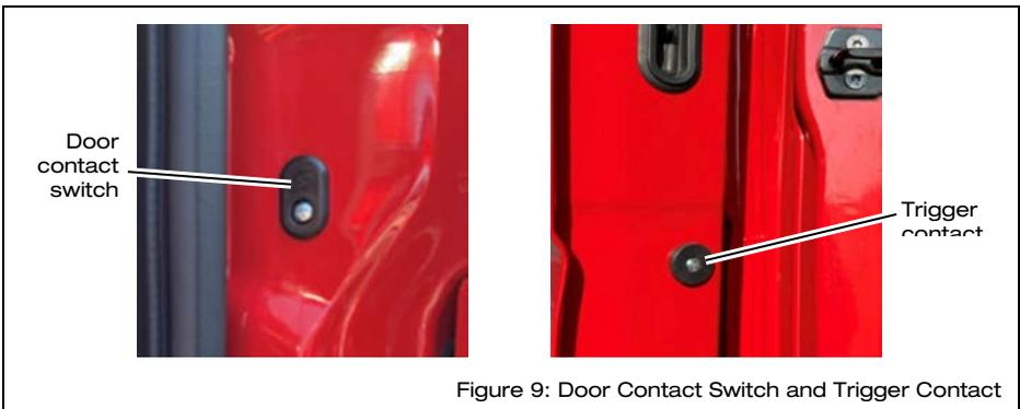
Figure 9: Door Contact Switch and Trigger Contact
