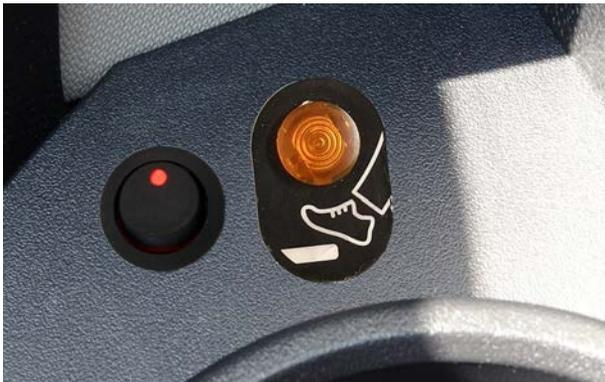
Figure 11: Deactivation Switch next to the Indicator Lamp
