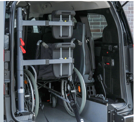
Optional the vehicle can be equipped with the head and backrest FUTURESAFE 2.0.
