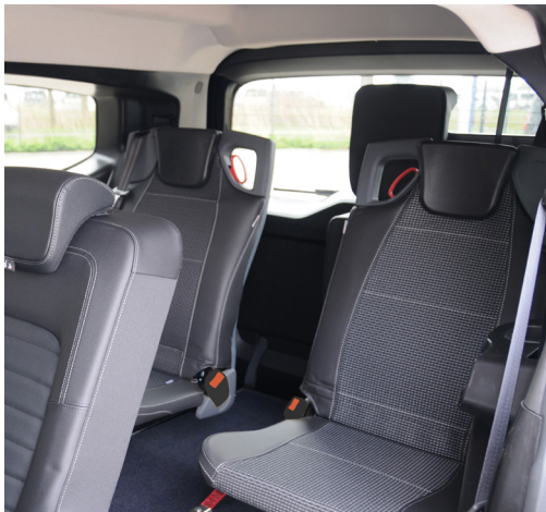
Optional tip & fold seats in 3rd row allow flexible use of the vehicle.
