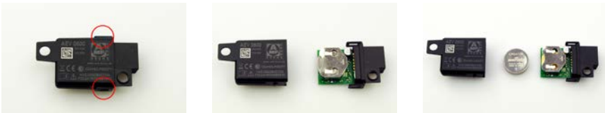
Figure 6: Opening the Transmitter Unit and Removing the Battery
