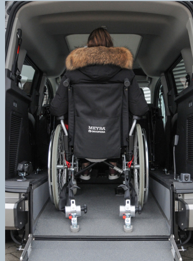
Rear attachment of the wheelchair using retractors
