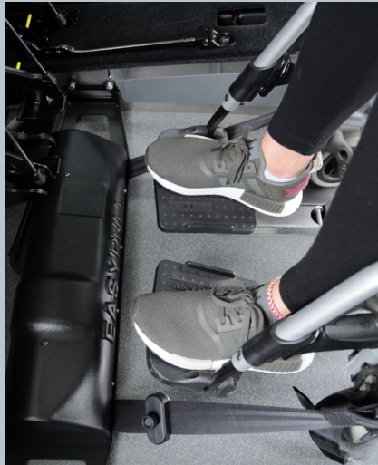
Fully integrated restraint system for the front wheelchair attachment
