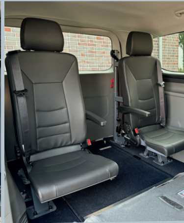
Optional tip & fold seats in third row allow flexible use of the vehicle.
