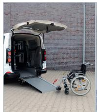
With the unfolded ramp the vehicle can be accessed comfortably with a wheelchair.
