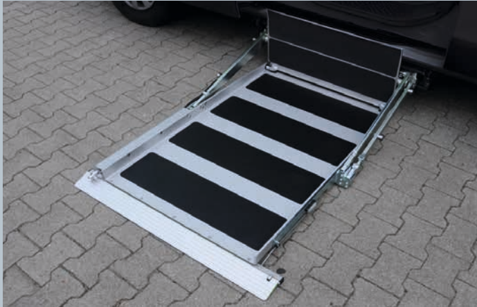
The lateral access with the flat side edge of the lifting platform saves space when driving up with the wheelchair.
